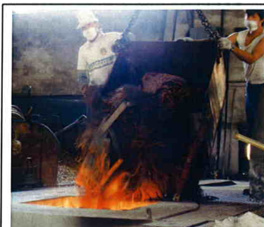
Fig 5 Feed Hooper for use with Overhead Crane
