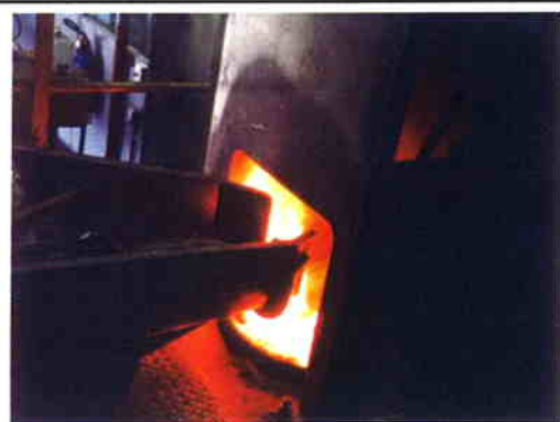
Fig 4 Vibrating Table feeding Swarf into Furnace
