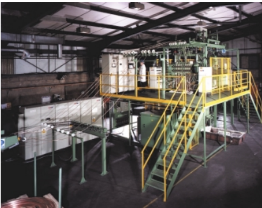
▼ Model RS 3000/8/8 copper rod casting machine - 6,000t./year
