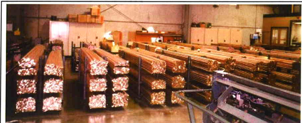
Fig 14 Typical Storage Rack Arrangement for Brass Rod
