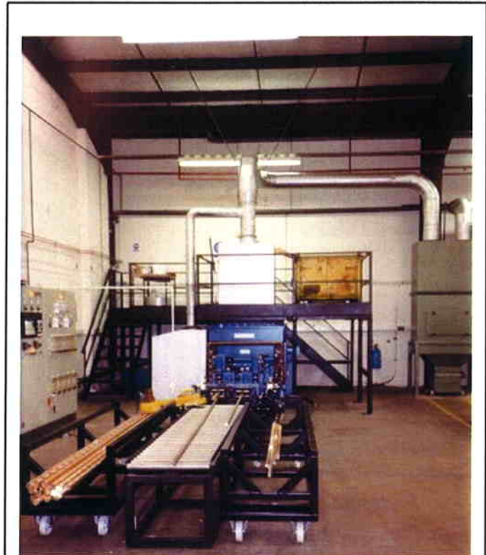
Fig 10 Rautomead Brass Rod Casting Installation. Note Fume extraction Hoods and hand Held Powered Bandsaw
