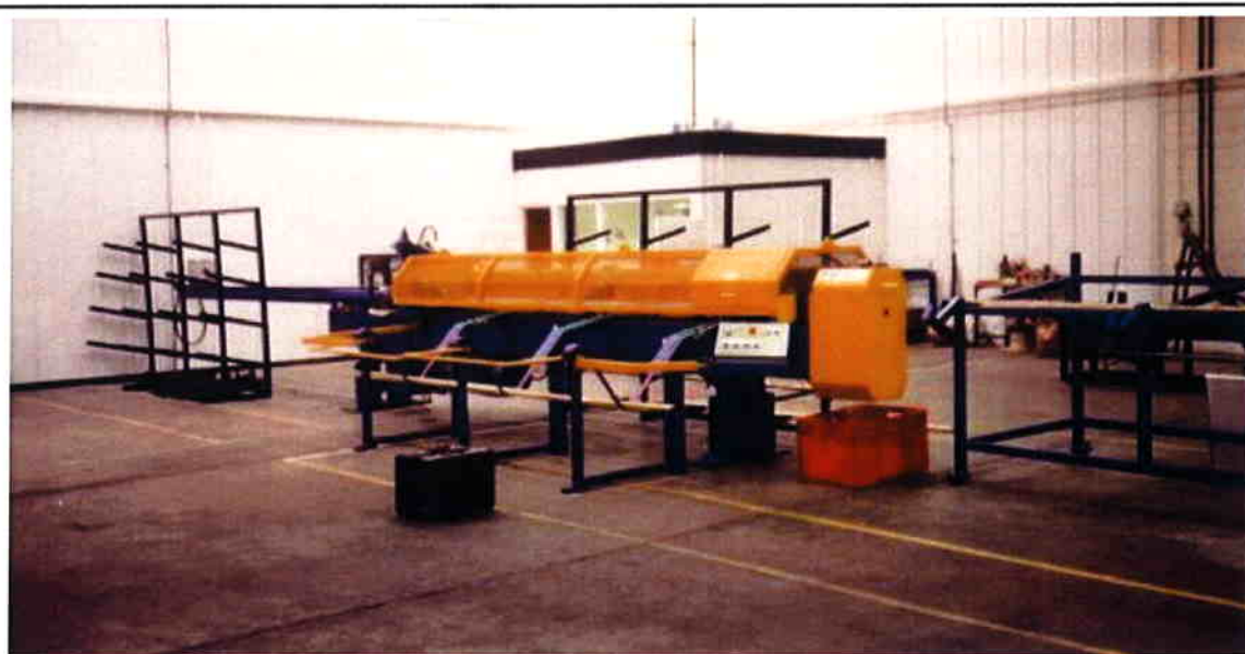
Fig 12 30 Tonne Hydraulic Shave Bench
