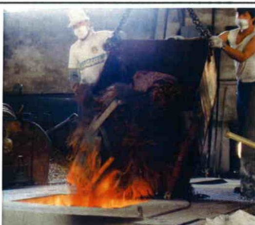
Fig 5 Feed Hooper for use with Overhead Crane
