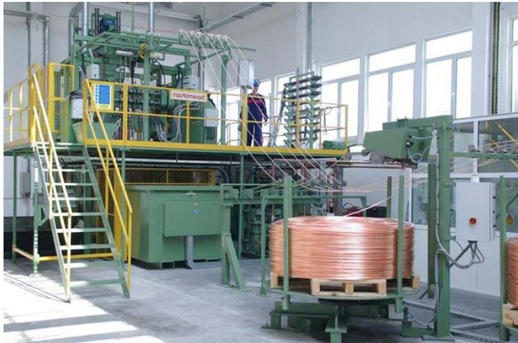
Fig. 1 Rautomead RS 3000 Copper Rod Casting Machine
