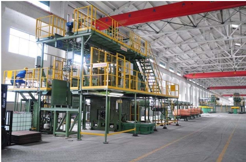
Fig. 9 Rautomead RS 3000/5-Cu-Mg Casting Machine
