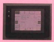
With the new RMK series, operators can view trends onscreen in any selected four from nine production parameters, magnify for close up detail and choose from thirty pre-set production recipes. A 24-hour operating clock is also part of the standard package.
